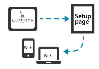
The Elertus Wi-Fi network cannot provide an internet connection, but will provide access to the SAFELERT setup web page.
