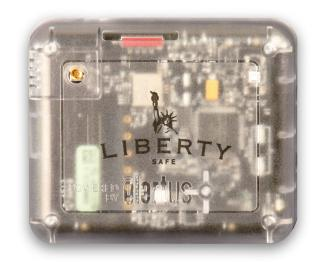
Install the batteries into your SAFELERT Sensor, and wait for the LED light to turn solid **RED**.
